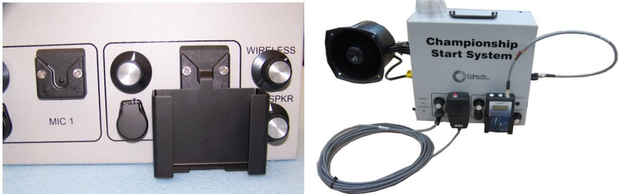
Attach the cable and adapter between the Dolphin Starter and the Timer Start jack on the ChampStart. **NOTE:** you must **unlock** the locking mini BNC connector when disconnecting from the Dolphin Starter or you will damage your cable.
