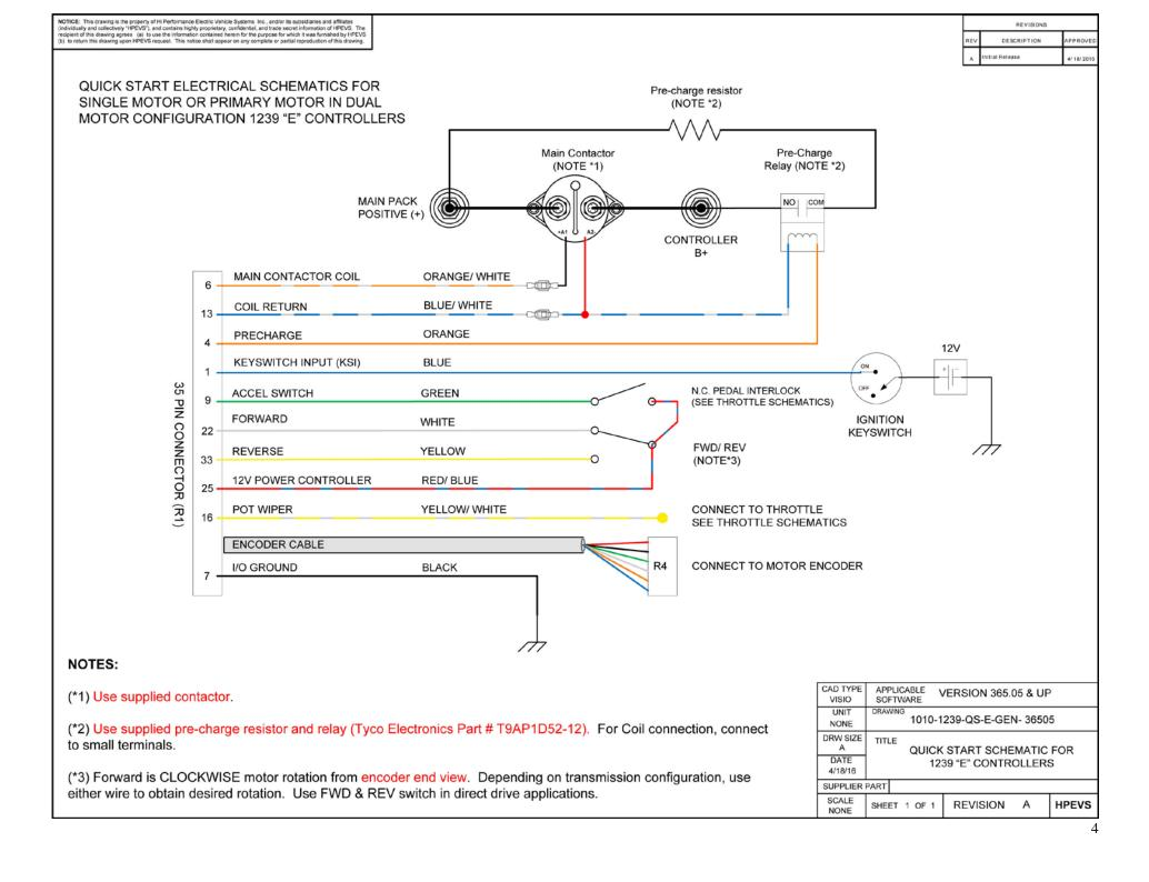
Quick Start Electrical Schematic Generic Software Pin Out Specific for 1239 "E" Controllers Single Motor or Primary in Dual Motor Applications
