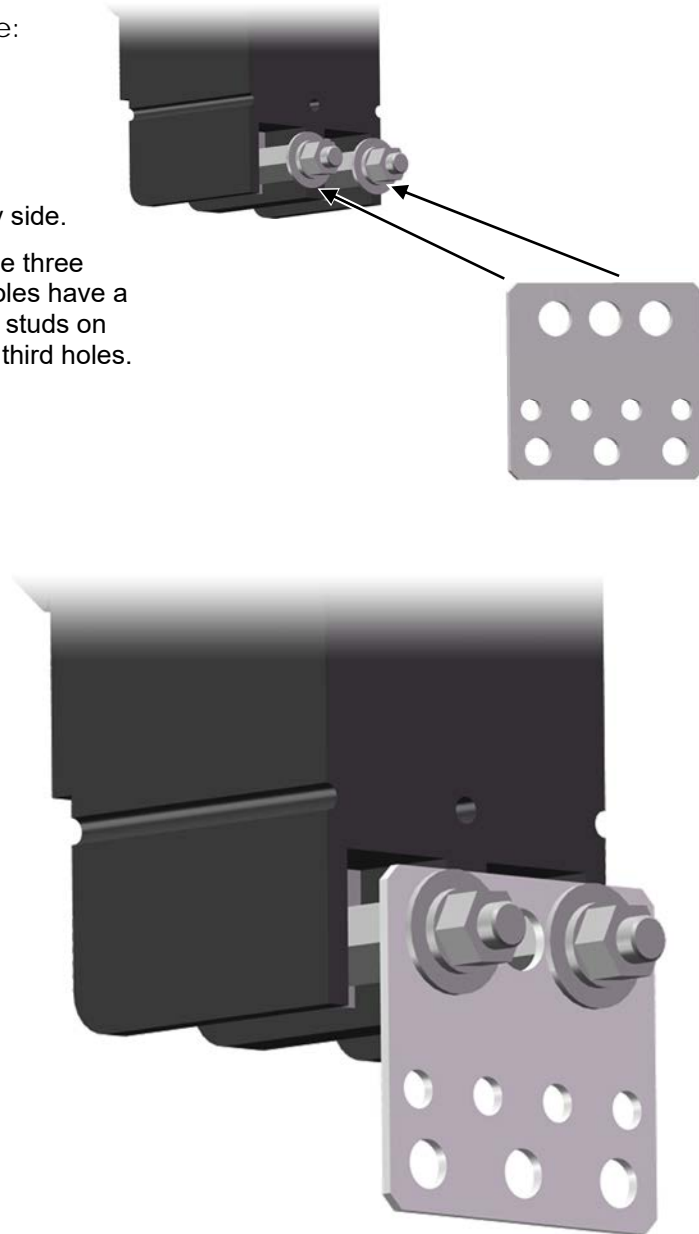
Figure 18 Assembling the DC Positive (+) Cable Plate
