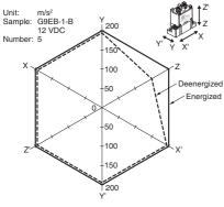
The value at which malfunction occurred was measured after applying shock to the test piece 3 times each in 6 directions along 3 axes.
